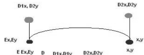
Figure 6. Bazier curve with directional point and starting point as well as ending point.
