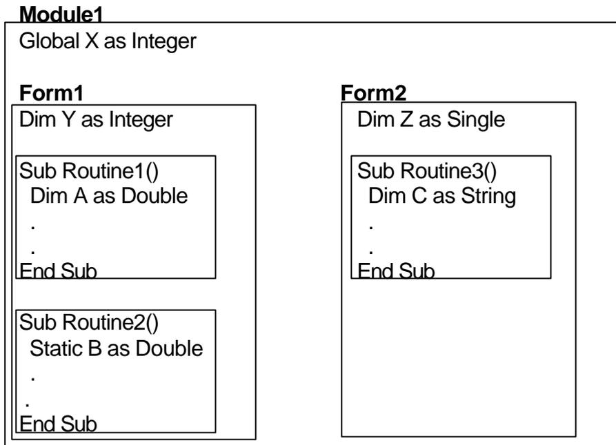
Procedure Routine1 has access to X, Y, and A (loses value upon termination)
