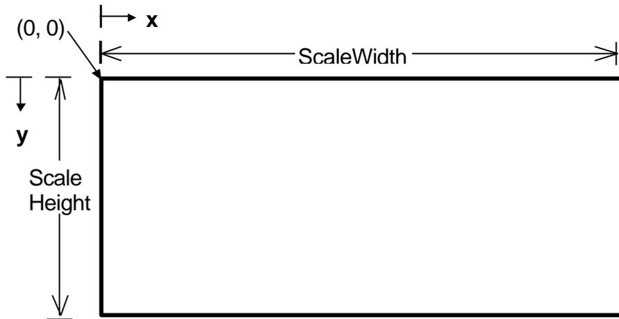
Note the **x** (horizontal) coordinate runs from left to right, starting at **0** and extending to **ScaleWidth - 1**. The **y** (vertical) coordinate goes from top to bottom, starting at **0** and ending at **ScaleHeight - 1**. Points in this coordinate system will always be referred to by a Cartesian pair, **(x, y)**. Later, we will see how we can use any coordinate system we want.
