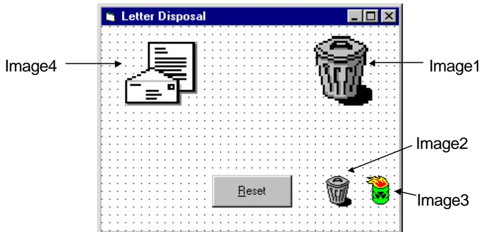
Some explanation about the images on this form is needed. The letter image is the control to be dragged and the trash can (at **Image1** location) is where it will be dragged to. The additional images (the other trash can and burning can) are not visible at run-time and are used to change the state of the trash can, when needed. We could load these images from disk files at run-time, but it is much quicker to place them on the form and hide them, then use them when required.
