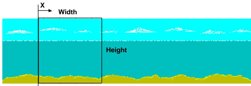
At each program cycle, we copy a bitmap of the size shown to a destination location. As X increases, the background appears to scroll. Note as X reaches the end of this source bitmap, we need to copy a little of both ends to the destination bitmap.
