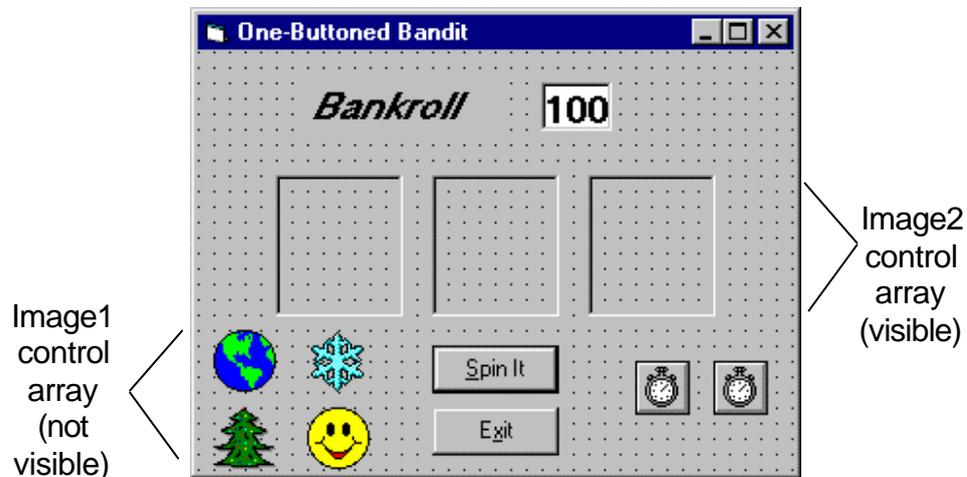
A few words on what we're doing. We will randomly fill the three large image boxes by choosing from the four choices in the non-visible image boxes. One timer (**timSpin**) will be used to flash pictures in the boxes. One timer (**timDone**) will be used to time the entire process.
