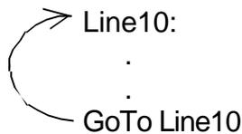
When the code reaches the GoTo statement, program control transfers to the line labeled Line10.
