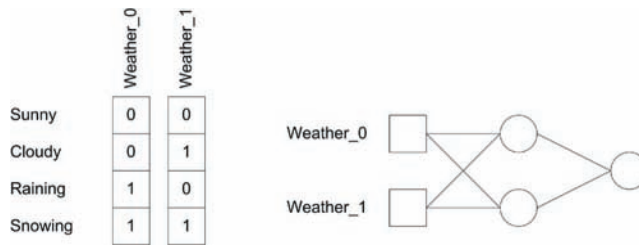
FIGURE 8.21: Using a binary encoding to reduce the number of inputs.
