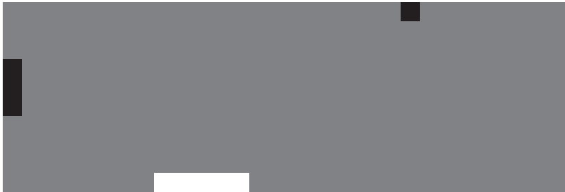
Figure 10.2.2 Initialized metal bar with black representing hot, white cold, and gray an intermediate temperature
