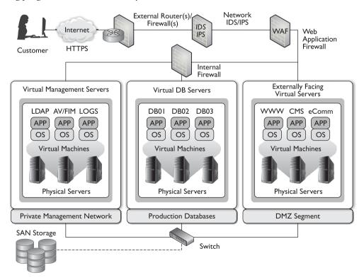
Figure 11-4 Segmenting virtual machines with firewalls
