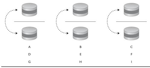
Figure 10-5 High performance striping with mirrored segments
