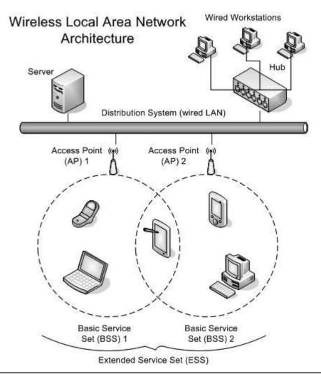
Figure 12-1 Example WLAN architecture
